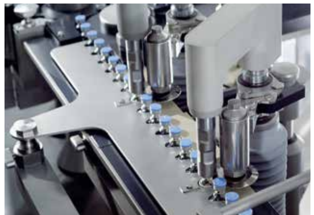
Integrated capping area
