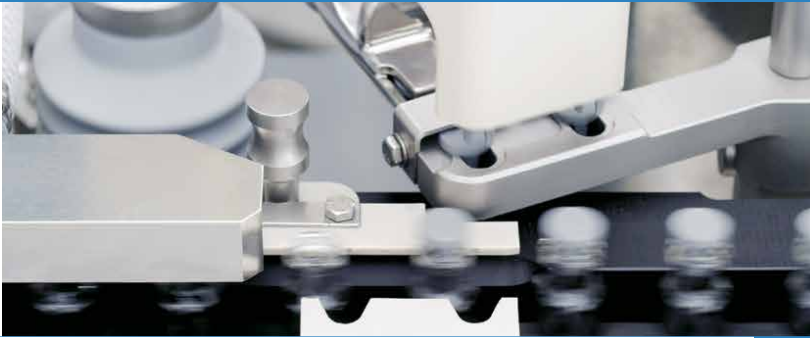
Nitrogen purging before stoppering station
