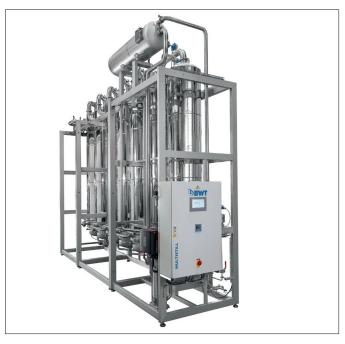
The BWT AQUA AG MS distillation units are designed to produce pharmaceutical grade Water for Injection (WFI) for the preparation of parenteral solutions, dilute samples in test laboratories, final flush in washers and similar applications. Water is produced by the evaporation, purification and condensation of feed water. MS units use the unique BWT AQUA AG internal preheating and separation systems for longer life and better performance.
